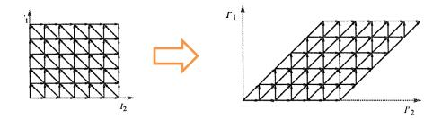
**Informal Definition:** Increase dependence distance by n by substituting loop index j with jj = j + n \* i.
